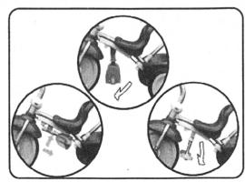
Put down foot rest, by sliding the top plastic section to the right then pulling the tube down as shown above. Finally unfold the foot rest. To fold up please reverse the above.
