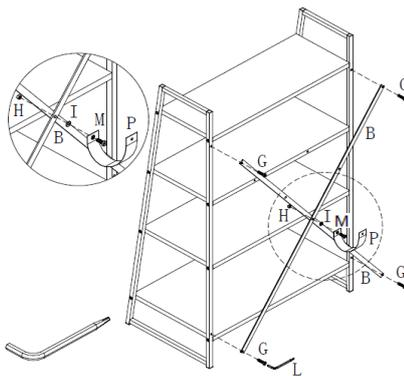
Step 5: Fasten the metal wire (Part B) and Board (Part D) with screws (part J).
