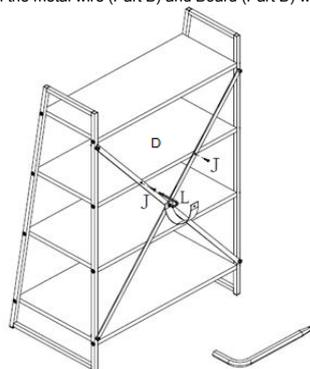
Step 6: Put screw (Part N) into the small hole of nylon tie (Part P) and across plastic anchor (Part O) to fasten to the wall. Fasten all screws firmly, assembly is now complete.
